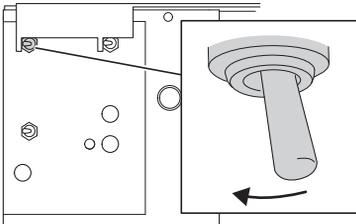
5. Place a 0.019" (0.05 mm) feeler gauge (B) between the lifting arm (C) and the flange (A) and make sure that the lifting arm completely meets the flange for about 1.5 seconds before it lifts again.
