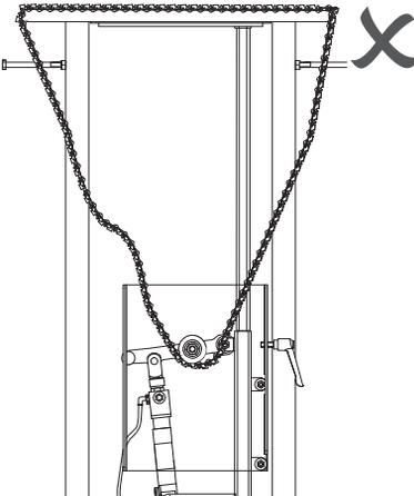
6. If the chain tension is too loose, repeat the procedure.
