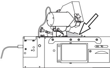
2. Make sure that the wires and when used with a stand, air hoses are correctly connected.
