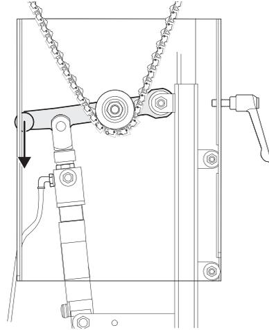
3. Move the tensioner downward until the chain is tightly secured in its position. There should be a gap of about 1/2" (12.7 mm) between the pneumatic-piston nut and pneumatic piston, where the piston should be visible.
