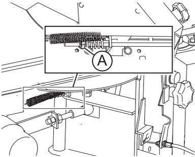
3. Do a sharpening test and make sure that the chain remains in its position during the test. See section 7.2, "Sharpening test."
