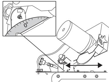
5. Change the grinding setting for the height of the depth gauges.
