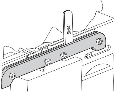
2. Turn the nut (A) in 1-1.5 turns clockwise, until the groove in the chain vise is  $0.070"$  (1.8 mm) to  $0.078"$  (2.0 mm) wide.
