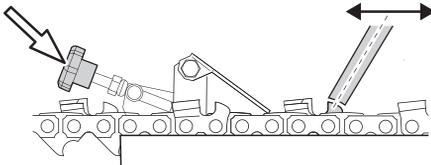
7. Make the grinding settings according to the manufacturer's recommendations.
