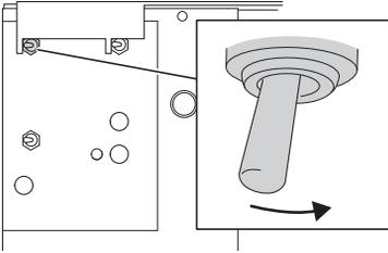
**⚠ Important!** If the chain has double-links, pull the chain back so that the grinding starts on the second double-link. If the chain has a joint with an irregular cutter sequence, start grinding behind it, to the left of the stop clamp.
