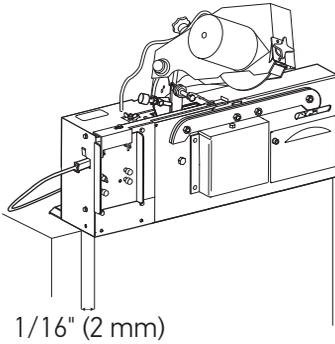
4. If the machines are not being used with the optional stand and the pneumatic tensioner, it should be used with the weight tensioner in order to provide the chain with the tension needed for grinding.
