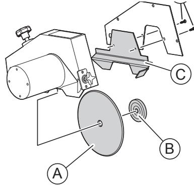
5. Remove the grinding wheel (A) from the grinding wheel axis and discard it in accordance with local, state, and national laws and regulations.
