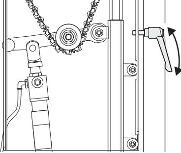
1. Lift the tensioner arm (there is a quick release function) and place the chain below the tensioner roll.
