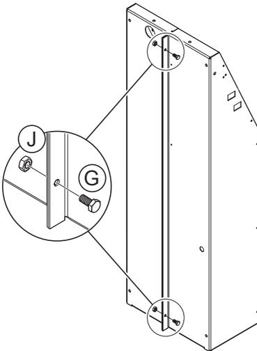
5. To complete the assembly of the stand, bolt the side support first to the base and then to the front piece.
