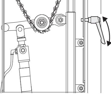
5. Gently press the chain with your hand to test the tension. The chain should not slacken.
