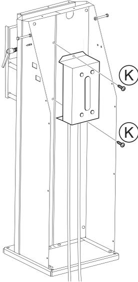
11. Next, place the machine on the stand. Fix it to the stand through the 3 holes located at the back of the machine with the bolts and nuts provided.
