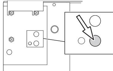
2. Set the grinding wheel switch to ON.
