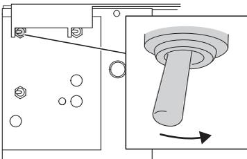
7. To set the wire so that the lifting arm meets the flange:
