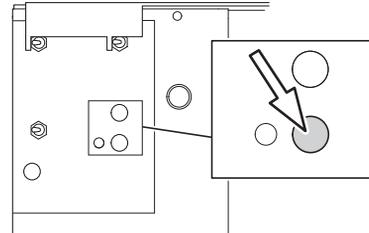
2. Press the grinding head positioning button to turn the grinding head to the left.
