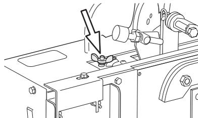
Note: Adjusting the pitch is not the same thing as adjusting the cutting tooth length (see number 13 below).
