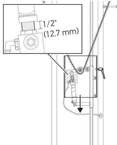
4. Tighten the locking handle to secure the chain.
