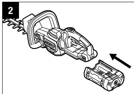
**NOTE:** Make sure that the latch on the hedge trimmer snaps into place and the battery pack is secured to the tool before beginning operation.
