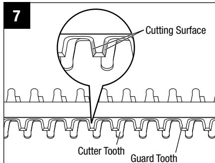
**NOTE:** Do not operate your hedge trimmer with dull or damaged cutting blades. This may cause overload and will give unsatisfactory cutting results.
